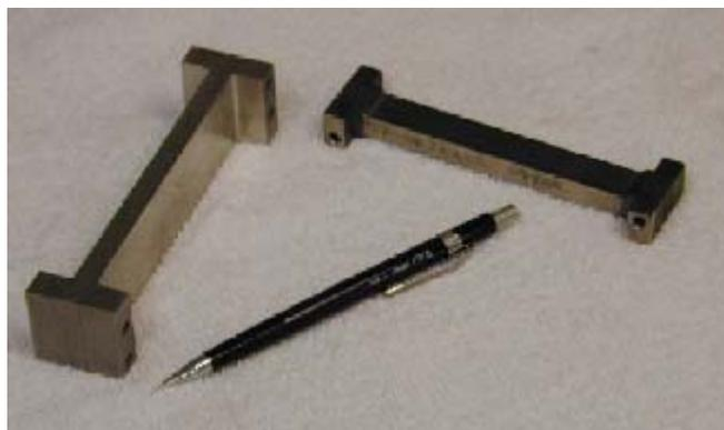
**Figure 8. Evaporator (left) and solution recuperator (right) used in the 250 Watt ammonia-water breadboard.**
