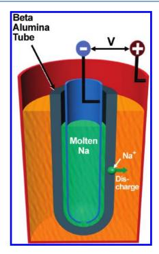
Figure 18. Single-cell and tubular design of a Na-beta battery. 10,180
