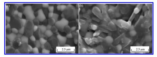
Figure 22. SEM images of (a) α-Al<sub>2</sub>O<sub>3</sub> and (b)  $\beta''$ -Al<sub>2</sub>O<sub>3</sub>. The  $\beta''$ -Al<sub>2</sub>O was obtained via the vapor phase conversion process by heat treating α-Al<sub>2</sub>O<sub>3</sub> at ~1450 °C in air for 2 h in  $\beta''$ -Al<sub>2</sub>O<sub>3</sub> packing powders. <sup>208</sup>
