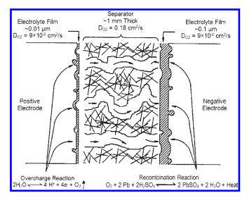
Figure 31. Construction of Sealed or VRLA, and conceptual view of internal oxygen cycle in a VRLA cell. $^{305}$
