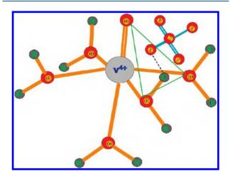
**Figure 11.** Schematic view of vanadyl ion with sulfate anions occupying second coordination sphere of the hydrated vanadyl ion. The dashed line represents the formation of new hydrogen bonds leading to proton exchange between sulfate anion and equatorial water molecule. <sup>51</sup>
