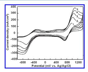
**Figure 13.** Cyclic voltammogram obtained at a glassy carbon electrode in 1 M VOSO<sub>4</sub>-2 M H<sub>2</sub>SO<sub>4</sub> solution; scan rates: (1) 100, (2) 200, (3) 300, (4) 400, and (5) 500 mV s<sup>-1</sup>.<sup>68</sup>
