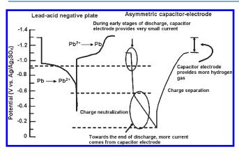
**Figure 34.** Operational potentials of a lead-acid negative plate and a carbon-based capacitor electrode during discharge and charge. <sup>309</sup>
