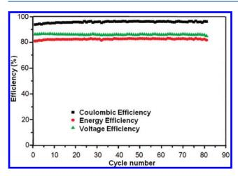
**Figure 16.** The cycle performance for a VRB single cell with a SPEEK/ TPA/polypropylene (PP) membrane at the current density of 35.7 mA/ cm<sup>2</sup>. Carbon felt with an active area of 28 cm<sup>2</sup> served as electrode materials for both negative and positive sides. The negative and positive electrolytes consisted of 1.5 mol  $L^{-1}$  VOSO<sub>4</sub> in 2.0 mol  $L^{-1}$  H<sub>2</sub>SO<sub>4</sub>. <sup>130</sup>
