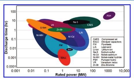
Figure 6. Power ratings and discharge times (i.e., energy ratings) of varied technologies 23,24 (Courtesy of Electrical Storage Association (ESA)).
