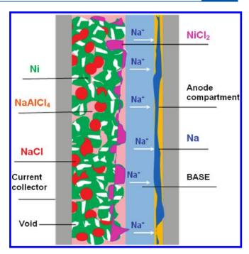
Figure 20. Schematic of cell structure and Na<sup>+</sup> transport during a charge process in Na-metal halide battery.
