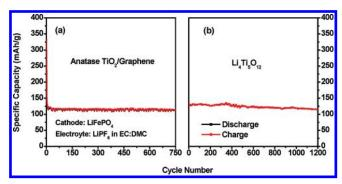
**Figure 30.** Cycling performance of Li-ion batteries made from LiFePO<sub>4</sub> cathode and (a) self-assembled anatase anode and (b)  $\text{Li}_4\text{Ti}_5\text{O}_{12}$  anode. <sup>280,298,300</sup>
