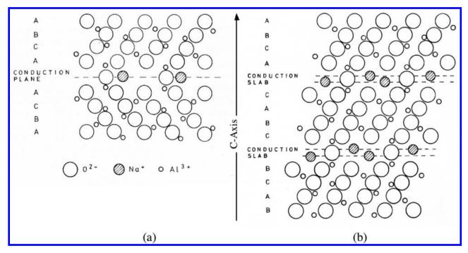
**Figure 21.** Projection of (a)  $\beta$ - and (b)  $\beta''$ -alumina unit cells on  $(11\overline{2}0)$  showing stacking sequence. <sup>179</sup>
