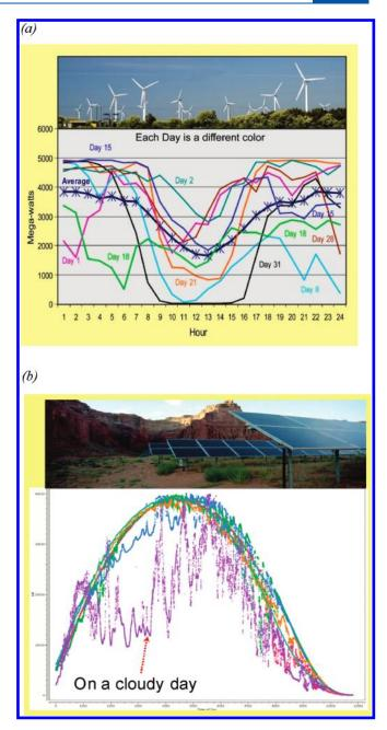
**Figure 1.** (a) Daily profiles of wind power projected by  $7 \times$  output in April 2005 for the year 2011 in Tehachapi, California (Courtesy of ISO California). (b) 5 MW PV power over a span of 6 days in Spain (Courtesy of AES).
