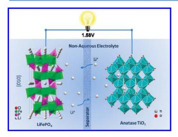
Figure 29. Li-ion batteries made from "zero" straining electrodes.
