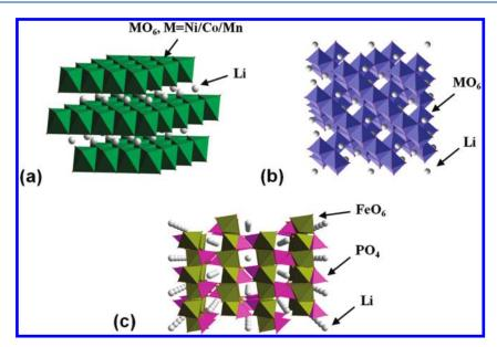
Figure 28. Structures of cathode materials: (a) Layered structure (LiMn<sub>x</sub>Ni<sub>y</sub>Co<sub>z</sub>O<sub>2</sub>); (b) spinel structure (LiMn<sub>2</sub>O<sub>4</sub>); (c) olivine structure (LiFePO<sub>4</sub>).
