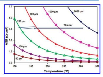
Figure 24. Area specific resistance ( $\Omega$  cm²) of  $\beta''$ -Al<sub>2</sub>O<sub>3</sub> as a function of temperature and thickness of the samples. The resistance was measured by AC impedance using a sodium—sodium cell configuration (both electrodes are sodium).
