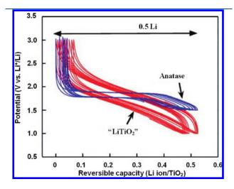
**Figure 26.** Comparison between the electrochemical behavior of rutile-(nanorod) and anatase type  ${\rm TiO_2}$  after the first reduction in a galvanostatic mode with 30 mA/g between 3 and 1 V in 1 M LiPF<sub>6</sub>. EC/DMC electrolyte at 20 °C. <sup>279</sup>
