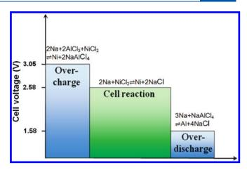
Figure 23. Cell reactions in sodium—nickel chloride battery at 300 °C. 180
