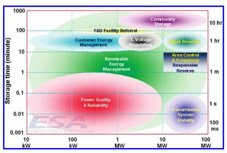
Figure 4. Power and discharge duration (or energy) requirements for varied applications<sup>20</sup> (Courtesy of Electricity Storage Association [ESA]).
