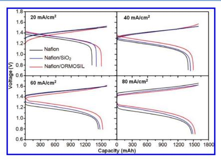
Figure 15. Charge—discharge curves of VRB with Nafion, Nafion/SiO $_2$ , and Nafion/ORMOSIL hybrid membranes at different current densities. The charge capacity was controlled to be 1600 mAh, corresponding to a redox couples utilization of 75%. Mixtures of 40 mL of 2 M V $^{3+}$ /V $^{4+}$  and 2.5 M H $_2$ SO $_4$  solutions were used as the starting anolyte and catholyte. <sup>82,118</sup>
