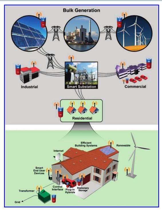
Figure 2. Schematic of applications of electricity storage for generation, transmission, distribution, and end customers and future smart grid that integrates with intermittent renewables and plug-in hybrid vehicles through two-way digital communications between loads and generation or distribution grids.<sup>10</sup>
