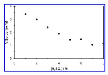
**Figure 9.** Dependence of the solubility of the V(IV)- $H_2SO_4$  solution on the  $H_2SO_4$  concentration at 25 °C.<sup>47</sup>
