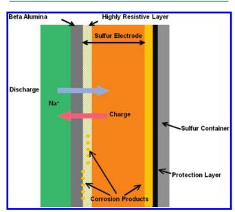
Figure 19. Schematic of cell structure and Na<sup>+</sup> transport during charge and discharge in an Na<sup>-</sup>S Battery (Courtesy of NGK Insulator, Inc.).
