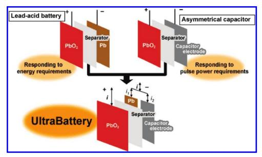
**Figure 33.** Schematic of an ultrabattery that integrates a lead-acid battery and lead—carbon asymmetric supercapacitor into a single unit<sup>320</sup> (Courtesy to The Furukawa Battery Co., Ltd.).
