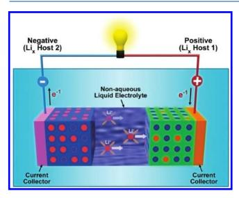
**Figure 25.** Schematic of a traditional Li-ion battery cell in which, during discharge, Li<sup>+</sup> ions migrate through the electrolyte, and electrons flow through the external circuit, both moving from the anode (negative) to the cathode (positive).
