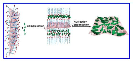
Figure 27. Schematic drawing of self-assembly of anatase TiO<sub>2</sub>/graphene nanocomposite. <sup>280</sup>
