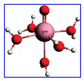
Figure 10. Structure of hydrated form vanadyl ion  $VO^{2+}$  in noncomplexing acidic solutions.  $^{48-51}$
