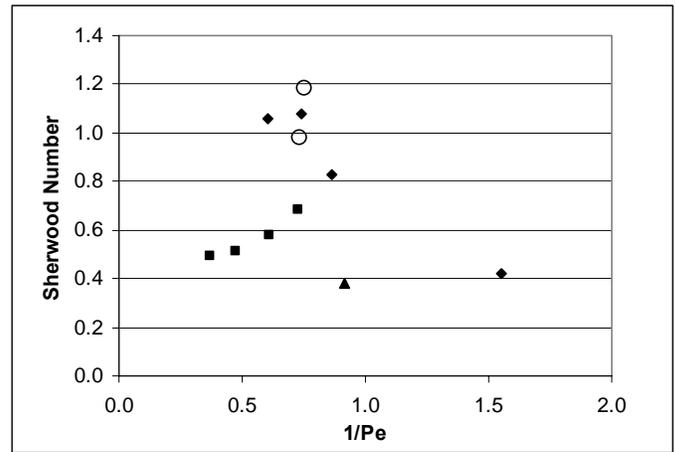
**Figure 5. Mass transfer in the Microwick absorber pre-prototype represented as the overall mean Sherwood number as a function of  $1/Pe$  with vertical flow at 1.3 bar, 10 wt% NH<sub>3</sub> feed and 21°C coolant air (◆); vertical flow at 1.6 bar, 22 wt% NH<sub>3</sub> feed, and 21°C coolant air (▲); side flow at 1.4 bar, 12 wt% NH<sub>3</sub> feed, and 50°C coolant air (■); and vertical flow at 5.4 bar, 29 wt% NH<sub>3</sub> feed, and 50°C coolant air (○).**
