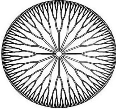
**Figure 1 - Microscale fractal-like branching desorber**
