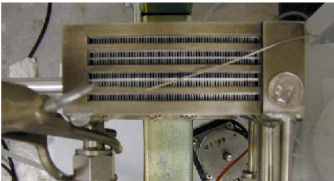
**Figure 4. Looking down on a prototype three-channel Microwick absorber with a dime included for perspective.**
