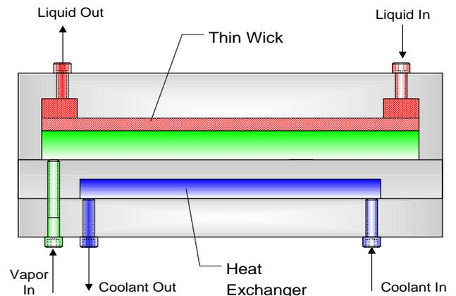
**Figure 2 - Schematic of a Microwick Absorber**
