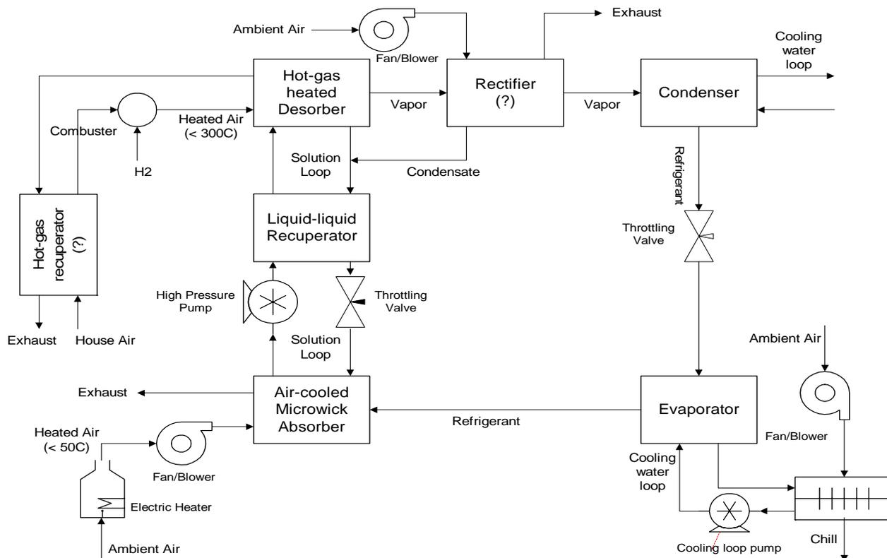
**Figure 7. Process flow diagram for 250 Watt ammonia-water heat pump breadboard.**
