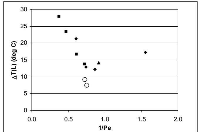
**Figure 6. Approach to equilibrium represented as the solution outlet temperature minus the saturation temperature for ammonia absorption as a function of  $1/Pe$  with vertical flow at 1.3 bar, 10 wt% NH<sub>3</sub> feed and 21°C coolant air (◆); vertical flow at 1.6 bar, 22 wt% NH<sub>3</sub> feed, and 21°C coolant air (▲); side flow at 1.4 bar, 12 wt% NH<sub>3</sub> feed, and 50°C coolant air (■); and vertical flow at 5.4 bar, 29 wt% NH<sub>3</sub> feed, and 50°C coolant air (○).**
